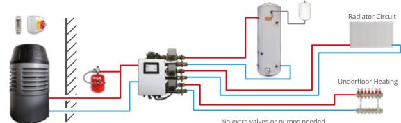
The RED heating system is not just a heat pump, RED want to control all the water moving in the house in harmony, so the RED system was designed to control all 3 parts of your heating system. You get a heat pump which contains a pump and flow meter, this connects to a RED low loss header.
